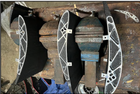
Laser-Cut Aluminium Reinforcements
