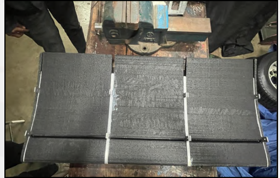
EPP Wing Panel and Aluminium Spars
