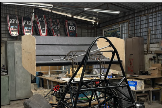
EPP Aero Integration on Car Chassis
