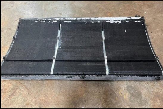
EPP Core with Carbon Fibre Skin
