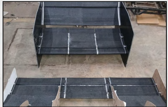
EPP Rear Wing Structure
